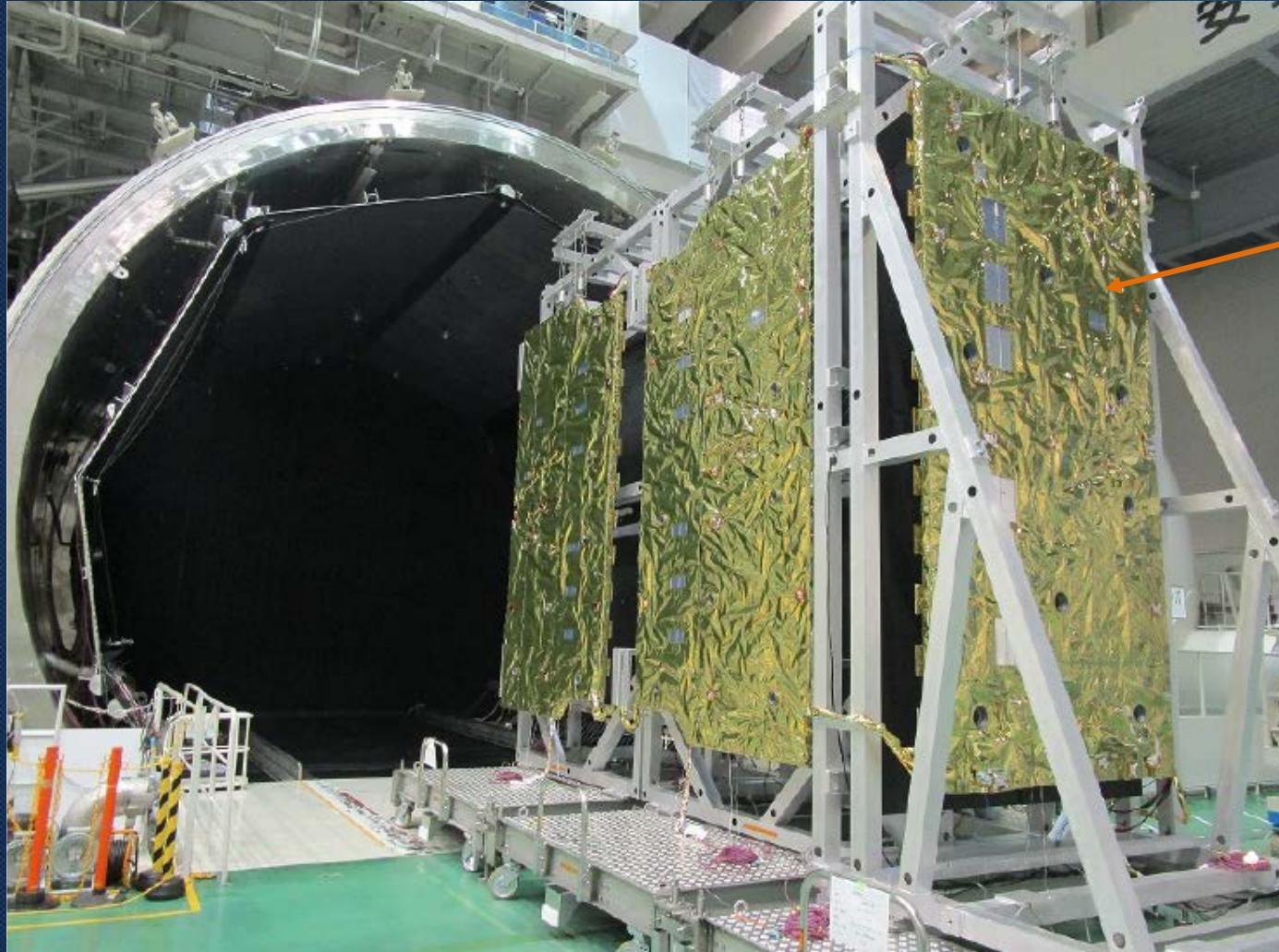
Proto-flight model of PALSAR-3 antenna
